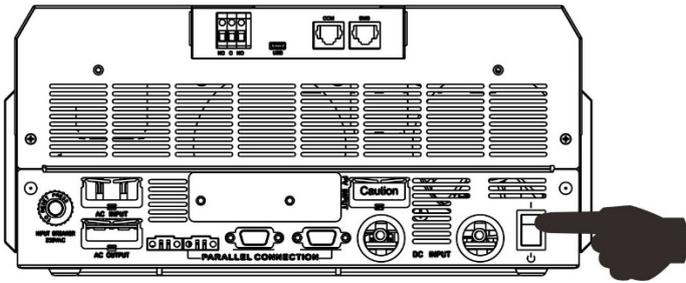
Step 4. Be sure to select battery type as "SOL" in LCD program 5.
