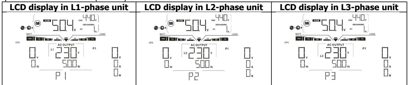
Step 4: Switch on all AC breakers of Line wires in AC input. If AC connection is detected and three phases are matched with unit setting, they will work normally. Otherwise, the AC icon will flash and they will not work in line mode.
