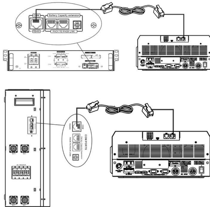
\* For multiple battery connection, please check battery manual for the details.
