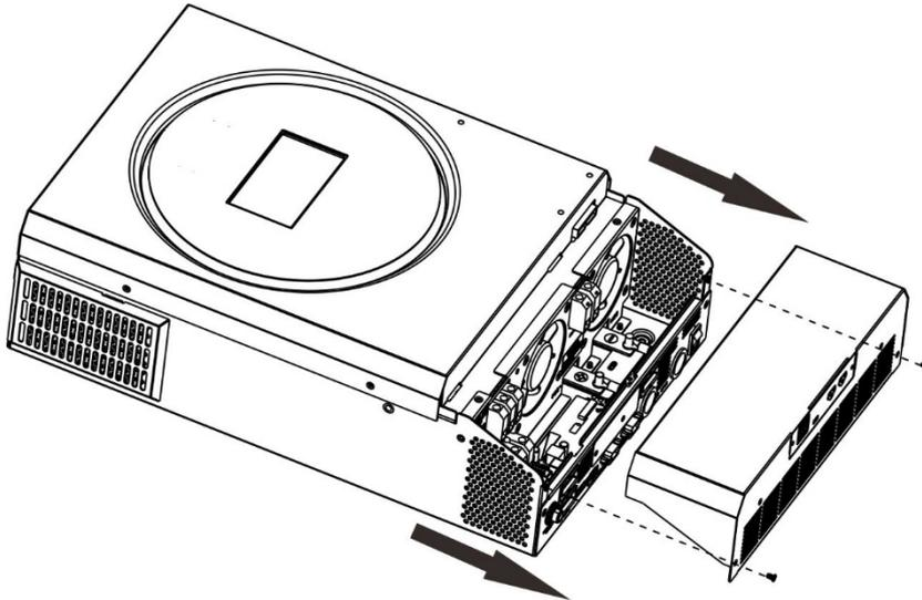
**Step 2:** Remove two screws as below chart and remove 2-pin and 14-pin cables. Take out the board under the communication board.
